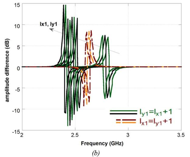
Fig. 3. (a) Amplitude of reflection coefficient for vertical and horizontal polarizations of an infinite array of 3-loop with stubs. (b) Amplitude difference between the reflection coefficients. The curves are obtained by progressively varying the length of the  $x$  and  $y$  directed stubs of the first loop and imposing  $l_{y1} = l_{x1} + 1$  or  $l_{x1} = l_{y1} + 1$ . The other stubs are fixed as:  $l_{x2} = l_{x3} = 2/64 D$ ,  $l_{y2} = l_{y3} = 4/64 D$ .
