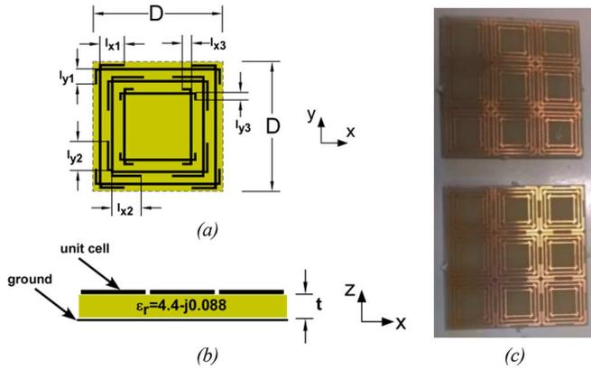
Fig. 2. (a) Unit cell geometry of the periodic surface-based chipless RFID, (b) side view of the proposed chipless tag, (c) chipless RFID prototypes.
