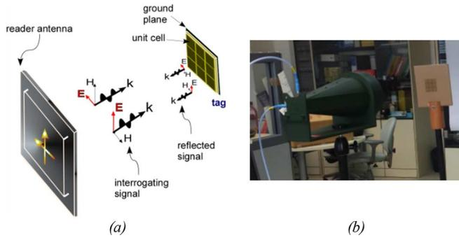
Fig. 1. (a) Sketch of the interrogating mechanism of differential coded chipless tags. (b) Experimental setup.
