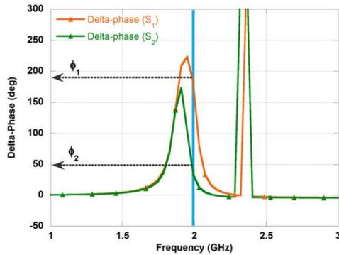
Fig. 3. Delta-phase response for the two stub lengths,  $S_1$  and  $S_2$ . Frequency  $f_1$  is highlighted in blue color.
