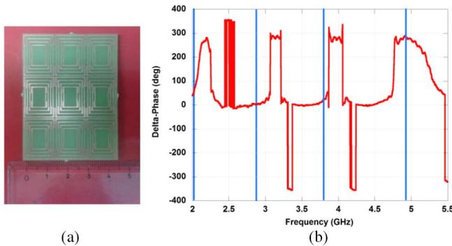
Fig. 9. (a) Prototype of the chipless RFID tag comprising  $3 \times 3$  unit cells and (b) quantized phase encoding (frequencies  $f_i$  are highlighted in blue).
