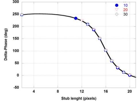
Fig. 4. Quantization of delta-phase at the fixed frequency  $f_1$  for different stub lengths. Pixels are defined as cell periodicity  $D_y$  over 64.
