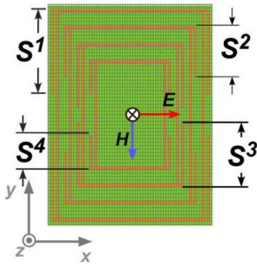
Fig. 6. Top view of the multiloop unit cell of the proposed periodic surface.
