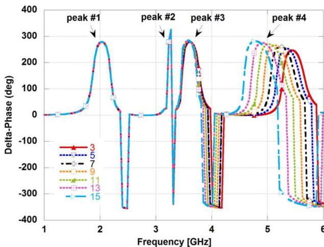
Fig. 7. Variation of the delta-phase response for a structure with the first three stubs fixed ( $S^1 = 12$ ,  $S^2 = 8$ , and  $S^3 = 7$ ) and the fourth spanning from 3 to 15 pixels.
