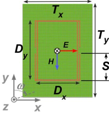
Fig. 1. Top view of the single-loop unit cell of the periodic surface. For a TE plane wave normally impinging on the surface, the electric field  $E$  is parallel to  $x$ -axis. The  $64 \times 64$  pixel grid employed by the PMM is shown as well. Angle  $\omega$  is measured with respect to  $y$ -axis.
