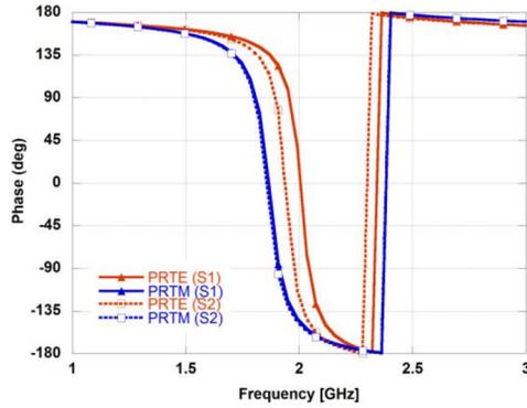
Fig. 2. Phase of the reflection coefficient for both a TE ( $PRTE$ ) and TM ( $PRTM$ ) plane wave incidence impinging on the periodic surface.
