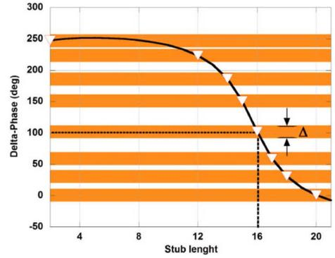
Fig. 5. Decision intervals of the quantized delta-phase defined by a fixed  $\Delta$ . In this case, a stub length = 16 produces a differential phase of  $100^\circ$ . The information is considered correctly retrieved if the measures delta-phase response is within  $[100^\circ - \Delta/2, 100^\circ + \Delta/2]$ .
