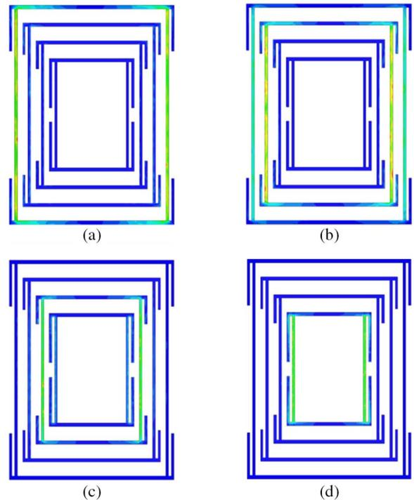
Fig. 8. Normalized current distribution at the resonance of (a) element#1 at  $f_1$ , (b) element#2 at  $f_2$ , (c) element#3 at  $f_3$ , and (d) element#4 at  $f_4$ .
