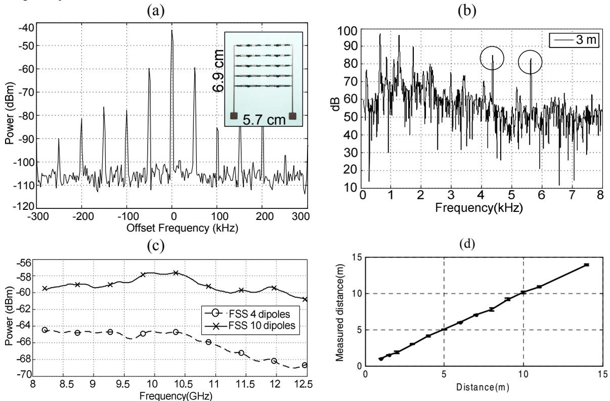
Fig.1: (a) Photograph of a FSS with 10 dipoles (arm length 6.25 mm, separation 7.5 mm). Measured spectrum at 10 GHz with the FSS modulated at 100 KHZ. (b) Base band output spectrum obtained with the FMCW radar at 3 m. (c) Comparison of the modulated power as function of the frequency for a FSS with 4 and 10 dipoles. (d) Measured distance and error as function of the distance.
