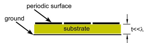
Fig. 1. Layout of the chipless RFID tag.
