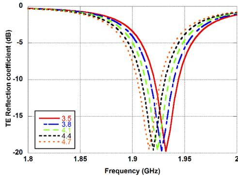
Fig. 2. Shift of the absorption peak as a function of the increasing CIM permittivity.
