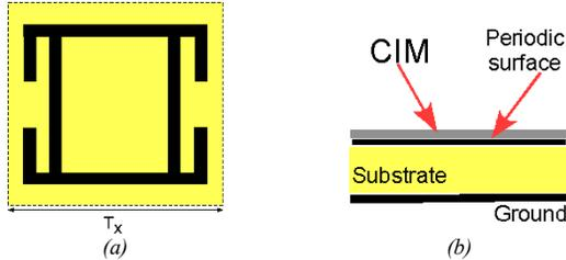
Fig. 1. Top view of the unit cell of the periodic surface a) and stackup of the employed configuration b).
