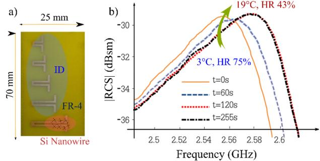
Fig. 3. a) Photograph of a chipless RFID tag integrating the sensor function. b) Influence of humidity on the EM response of a resonator containing a deposit of Si nanowire.
