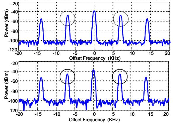
Fig. 2. Measurement of the spectrum at 10 GHz with a modulation frequency of 7 kHz at 90° of orientation. Transponder based on a dihedral corner reflector (top) and a cross reflector (bottom).
