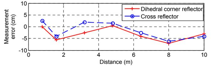
Fig. 6. Measured distance obtained from the dihedral corner reflector transponder (solid line) and the cross reflector transponder (dashed line).
