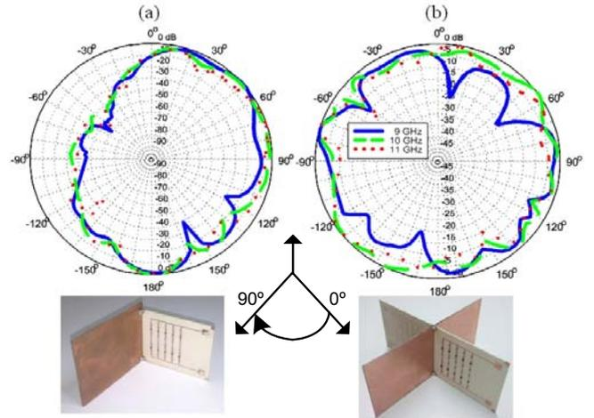
Fig. 3. Photograph and normalized measured power as a function of angle at 9, 10 and 11 GHz of (a) a dihedral corner reflector transponder and (b) the cross reflector transponder.
