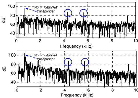
Fig. 4. Measurement of the dihedral corner reflector transponder (top) and a cross reflector transponder (bottom) at 3.2 m with  $f_m=5$  kHz modulation.
