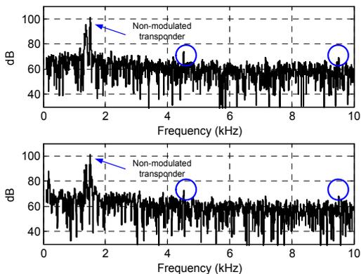
Fig. 5. Measurement of the dihedral corner reflector transponder (top) and a cross reflector transponder (bottom) at 10 m with  $f_m=7$  kHz modulation.
