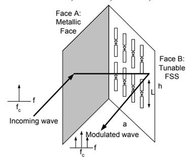
The diagram illustrates a corner reflector with two faces: Face A (Metallic Face) and Face B (Tunable FSS). An incoming wave with frequency  $f_c$  and angle  $\phi_c$  is incident on the corner. The angle between the two faces is  $\alpha$ . The distance from the corner to the FSS face is  $a$ , and the height of the FSS face is  $h$ . A modulated wave with frequency  $f$  is reflected from the FSS face. The scattered field is represented by the equation above.
