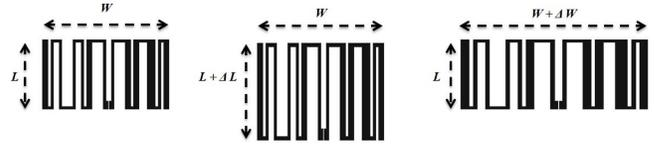
Fig. 1. Impedance matching based on the optimization of barcode dimensions: bar length ( $L$ ) and bar width ( $W$ ).
