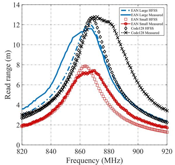
Fig. 4. Comparison between the read ranges of realized prototypes: HFSS simulations versus measurements.
