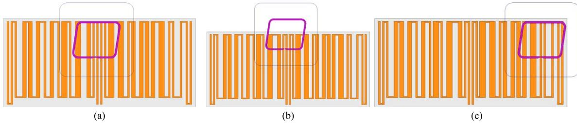
Fig. 5. Parametric study on the position of the AK tag. (a) Optimum performance as the AK tag is centered. (b) Weak coupling as the AK tag is shifted 5 mm away from the stubs. (c) Lower coupling as the AK tag is placed on the edge of the structure.
