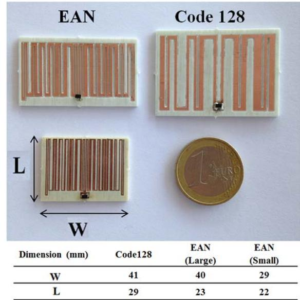
Fig. 3. Realized prototypes on Rogers RO4003 substrate. Code128 (right) and two different sizes of EAN (left).
