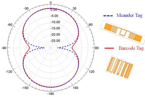
Fig. 2. Comparison between the simulated directivities of a conventional meander tag and the proposed barcode tag design.
