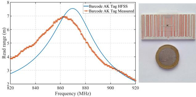
Fig. 6. Measured read range versus HFSS simulation of an AK tag coupled to EAN barcode at the optimum coupling position.
